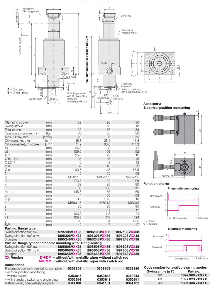
Clamping force diagrams and other accessories: see data sheet B 1.881. Further proximity switches: see data sheet B 1.552.
