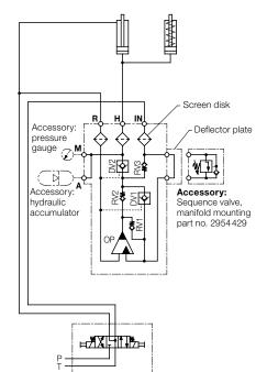
Power unit with a pressure filter 10 µm is required.
