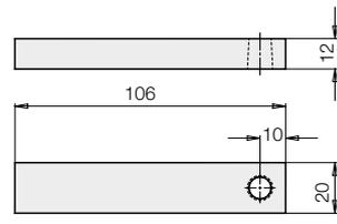
**Connecting dimensions for special clamping arms**
