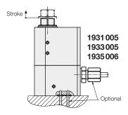
When pressurising the element, the support plunger extends with spring force against the workpiece. Locking then takes place automatically.
