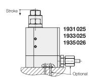
When loading the fixture, the support plunger is pushed back by the workpiece and makes contact with the workpiece by spring force. Hydraulic locking can then be initiated. During unclamping the support plunger will be unlocked and extends with spring force when the workpiece is removed.
