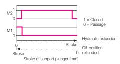
For process-safe functioning of position monitoring, air pressure and air volume must be adjusted.
