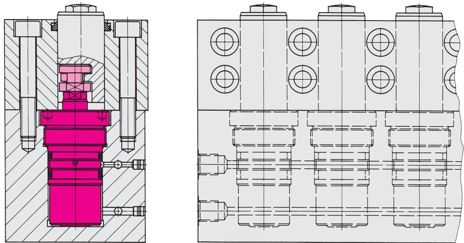
Double-acting threaded-body cylinders as pull-type cylinder for a multiple clamping fixture to mill a wrench flat
