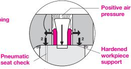
Clamping and unclamping monitoring
