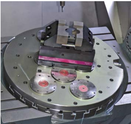
Workholding system HILMA.MCP Z with workpiece-specific base jaw and form jaw used on a 5-axis machining centre.
