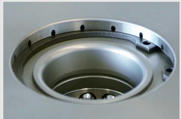
Openings for centre blow-out ducts
