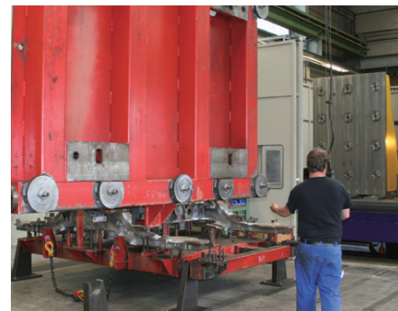
Wotan: machine table with right-angled clamping plate 1 and right-angled clamping plate 2. Loading is undertaken using the overhead crane. The „third hand function“ and optional clamping check are also an advantage during handling like the optical release check.
