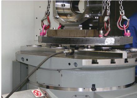
DMU 100: optical release check – „Thank heavens for hydraulics!“ The Speedys lift the pallet on release. Thus safe handling is guaranteed.
