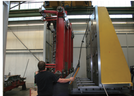
Wotan: machine table with right-angled clamping plate 1 and right-angled clamping plate 2. Loading is undertaken using the overhead crane. The „third hand function“ and optional clamping check are also an advantage during handling like the optical release check.
