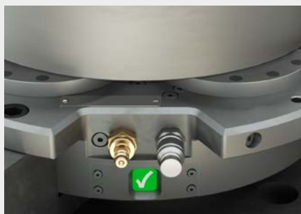
The green display shows that clamping is correct.
