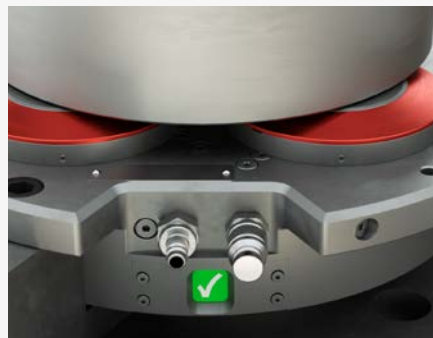
The green display shows that clamping is correct.
