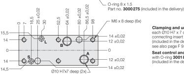
Clamping and unclamping each Ø10 H7 x 7 deep for connecting insert 9210132 (included in the delivery),
