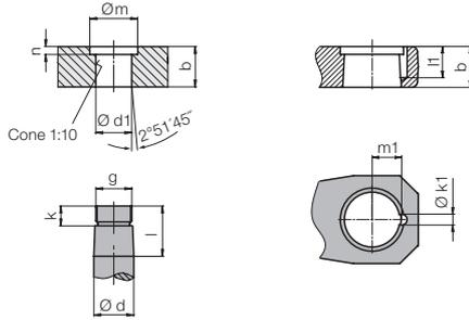
Clamping arm blank with indexing
