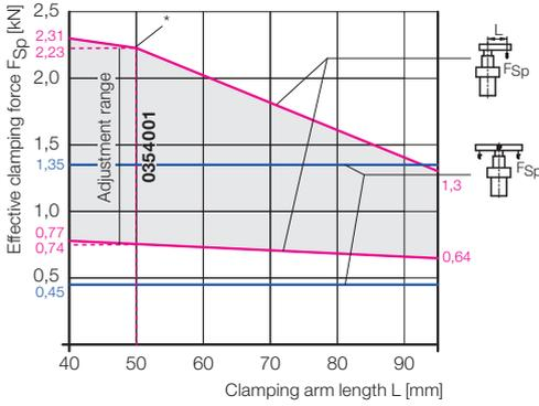
\* For clamping arm lengths > 50 mm, please observe the permissible setting parameters for the effective clamping force according to the operating instructions.
