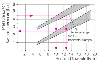
Required flow rate depending on the switching pressure of the pneumatic pressure switch for a pressure drop  $\Delta p$  2 bar
