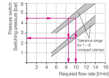
Required flow rate depending on the switching pressure of the pneumatic pressure switch for a pressure drop  $\Delta p$  2 bar
