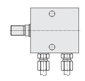
Manifold mounting versions with O-ring sealing
