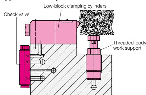
**Minimum pressure p<sub>Z</sub> for unblocking at pressure p<sub>A</sub> (p<sub>B</sub> = 0 bar)**
