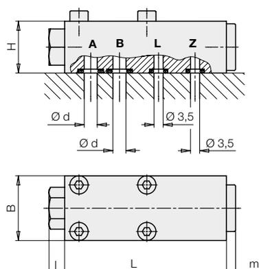
**Drilling pattern of the base plate**
