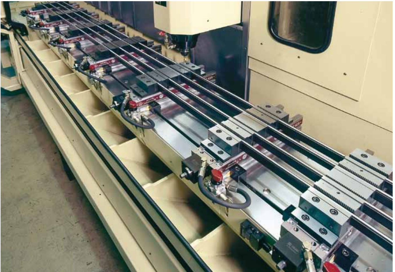
DS hydraulic arranged in a row for clamping of workpieces which require several clamping points. Can be automated.
