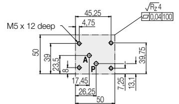
Manifold-mounting connection with hole pattern as per DIN 24340 form A 6, CETOP 4.2-4.3, ISO 4401
