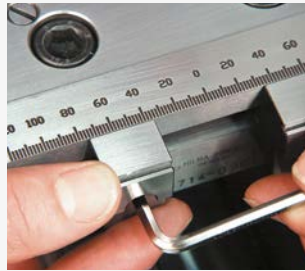
2. Set the outer edges of the inserts approx. 2mm below the finished dimension.
