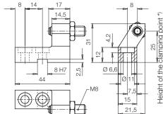
Clamping jaw for exterior clamping of a workpiece web with a thickness of 6 up to 14 mm (adjustable from 0 up to 18 mm).
