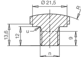
**Contact bolt for contact control**
