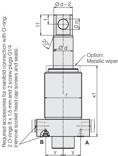
Required accessories for manifold connection with O-ring:
