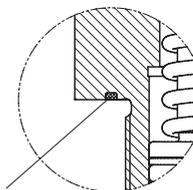
For piston  $\text{Ø } D = 32 \text{ mm}$  the knife edge will be replaced by a Kantseal joint.
