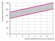
Chart valid for horizontal mounting position; for vertical arrangement, the weight of the clamping jaws must be taken into account.
