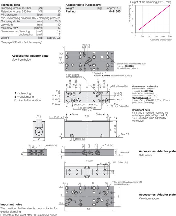
exterior clamping. Lubricate at the latest after 500 clamping cycles the clamping slide via the central lubrication. (Recommended: slide way oil ISO 68) Never use the complete clamping stroke to guarantee safe clamping of the workpiece. Max. operating temperature 80 °C.
