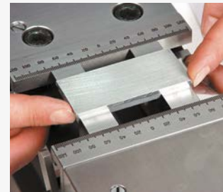
3. Insert workpiece blank centrally by sight and clamp
