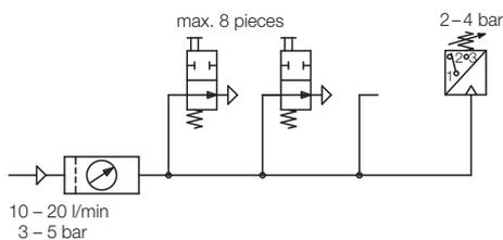
For the evaluation of the pneumatic pressure build-up, standard pneumatic pressure switches can be used. It is possible to monitor with one pressure switch up to 8 position monitorings connected in series (see circuit diagram). It has to be considered that process-safe functioning of pneumatic position monitorings is only guaranteed with throttled air and system pressure. The nominal values are indicated below technical characteristics.
