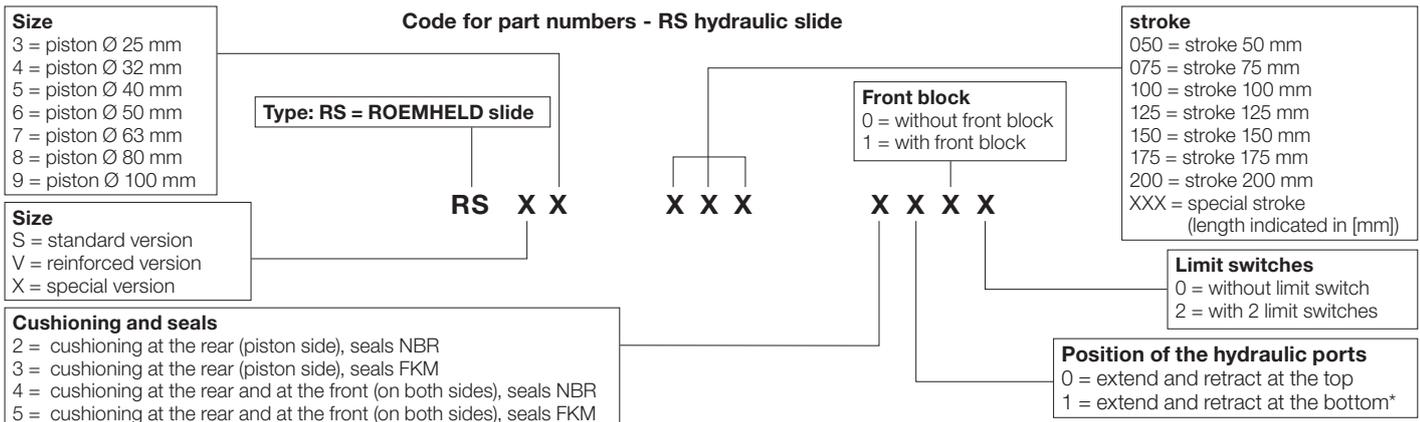
\*) Manifold-mounting connection at the front, pipe thread at the rear
