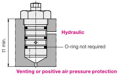
**2. Venting via drilled channels**
