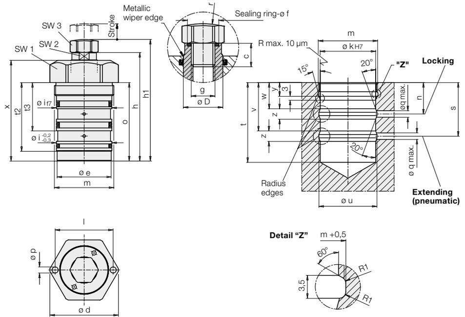
The support plunger contacts the workpiece by air pressure. The contact force is proportional to the air pressure less spring return force. The support plunger will be locked by hydraulic pressure and can compensate forces in axis direction.
