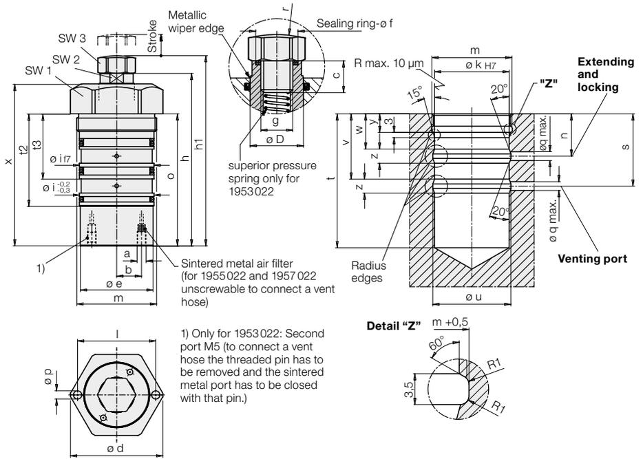
The support plunger is extended by a hydraulically pressurised small piston and contacts the workpiece with spring force. The support plunger will be locked by the increasing hydraulic pressure and can compensate forces in axis direction. For unclamping hydraulic pressure will be released. The small piston retracts by spring force to its off-position and also retracts the support plunger.
