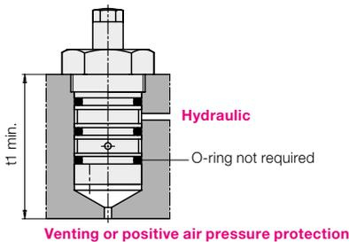
**2. Venting via drilled channels**
