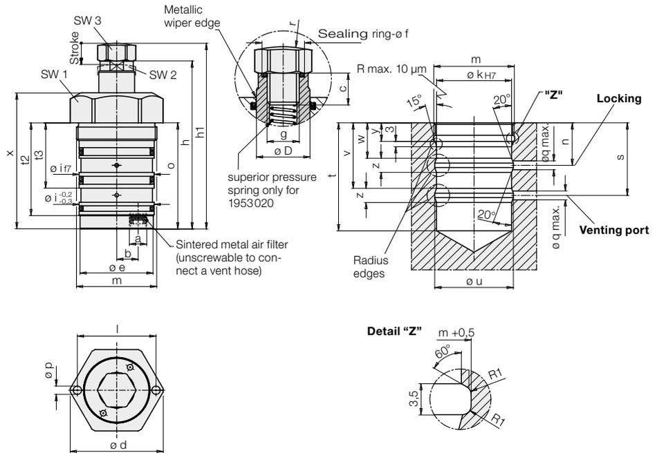
The support plunger is pushed back by the inserted workpiece, the spring force has to be overcome.
